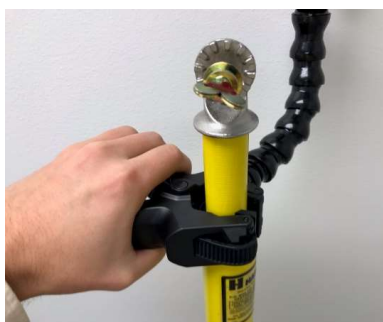
Sliding the GoPro® Camera into the camera mount
