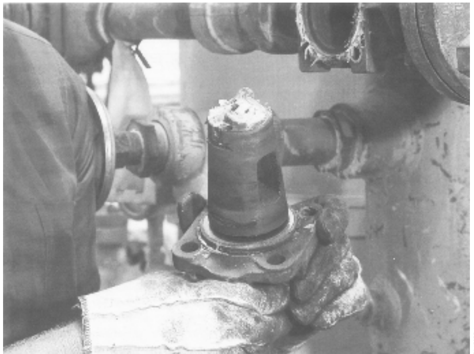
Valves protected by MOLYKOTE 3452 Chemical Resistant Valve Lubricant show no evidence of corrosion or degradation of lubricant.
